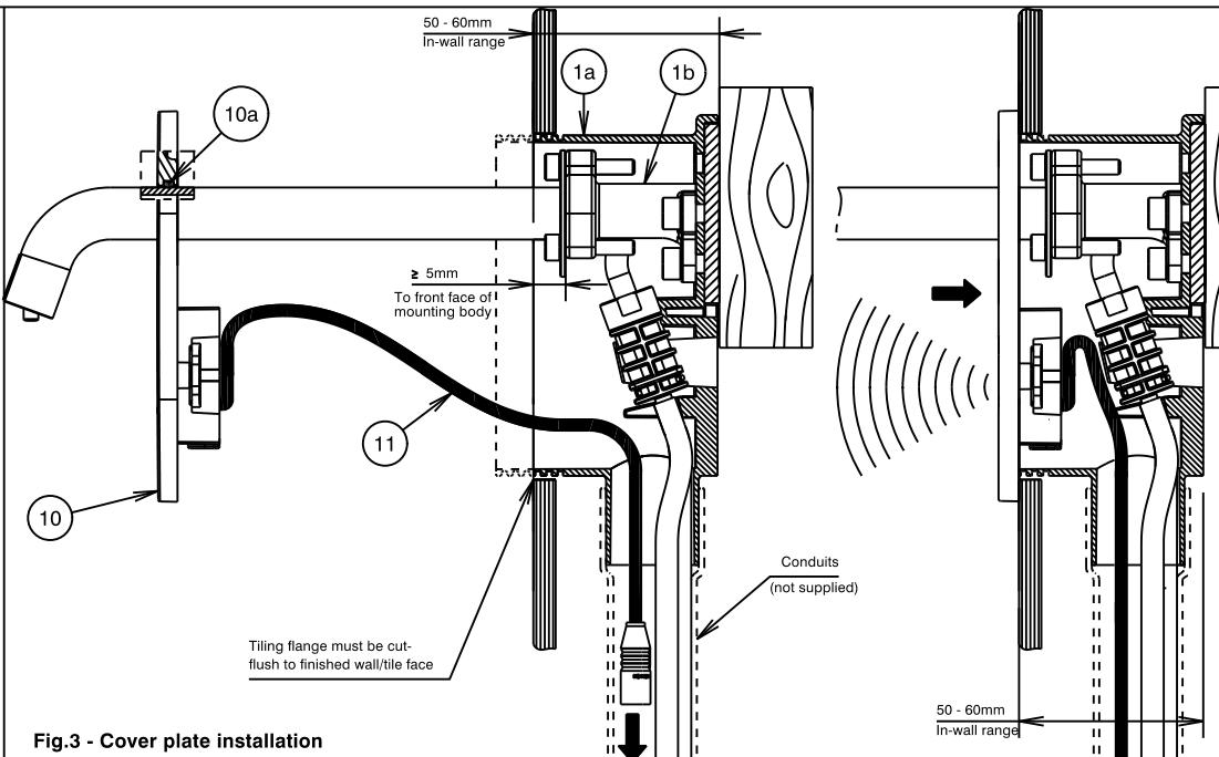
Fig.3 - Cover plate installation
